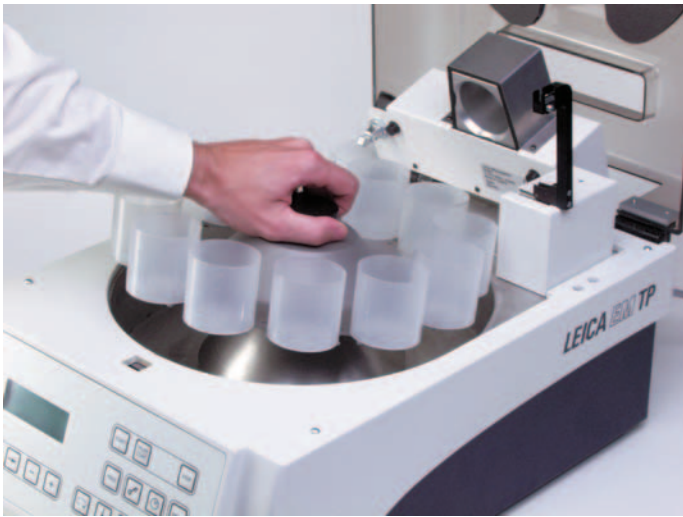
Moveable H/C unit for safe and easy access of carousel
