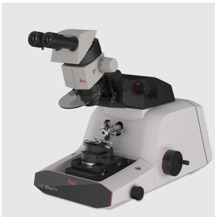
Basic - manual UC for sample sectioning in life and material sciences
