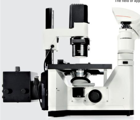
Leica DM IL LED with fluorescence axis and 3-position slider
